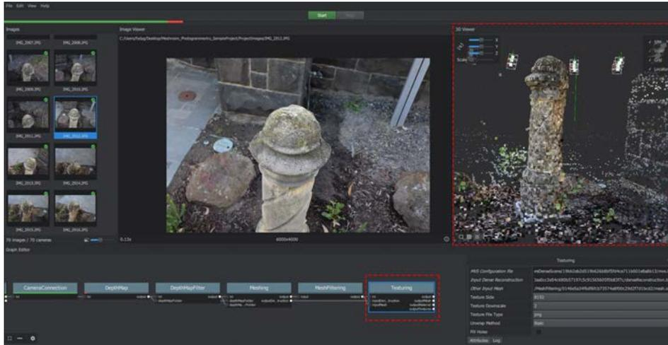
Figure 4. Creating a model of relay column through photogrammetry and the meshroom program, copy of <https://msd-makerspaces.gitbook.io>
